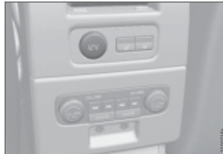
12 V socket in tunnel console, rear seat.
